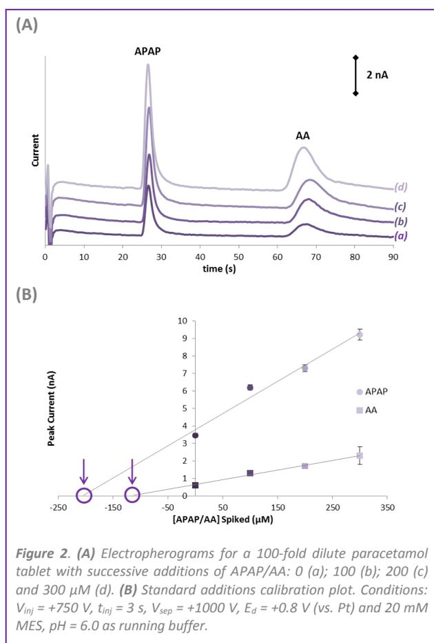
**Figure 2.** (A) Electropherograms for a 100-fold dilute paracetamol tablet with successive additions of APAP/AA: 0 (a); 100 (b); 200 (c) and 300  $\mu M$  (d). (B) Standard additions calibration plot. Conditions:  $V_{inj} = +750$  V,  $t_{inj} = 3$  s,  $V_{sep} = +1000$  V,  $E_d = +0.8$  V (vs. Pt) and 20 mM MES, pH = 6.0 as running buffer.
