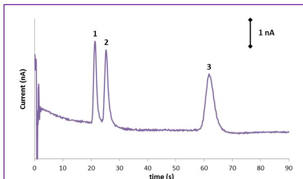
**Figure 1.** Electropherogram for a sample mixture of (1) *p*AP 100 µM, (2) APAP 200 µM and (3) AA 500 µM using a SU-8/Pyrex microchip with integrated Pt film end-channel detector. Conditions:  $V_{inj} = +750$  V,  $t_{inj} = 3$  s,  $V_{sep} = +1000$  V,  $E_d = +0.8$  V (vs. Pt) and 20 mM MES, pH = 6.0 as running buffer.
