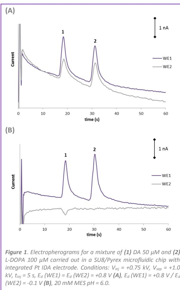
The separation of the two compounds is accomplished in less than **40 s**. Moreover, the use of an *interdigitated array* (IDA) electrode detector improves the benefits of microfluidic systems. In this case, each set of microelectrodes can be potentiostated individually, so that two analytical signals can be simultaneously recorded.
